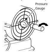
Figure 10 - Adjusting Pump Pressure
